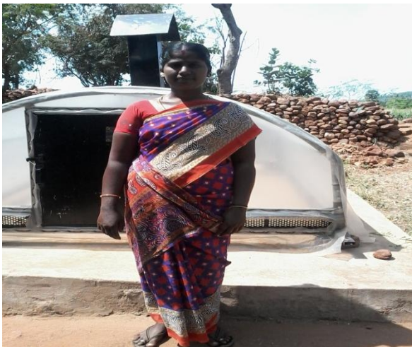
Smt. Poongodi standing in front of the drying plant installed with the help of technology disseminated by KVK very recently in her village. It is a privately made plant in which farmers can dry their medicinal plants, leaves, fruits etc. It is an organic way to get the things dry. Without losing its colour or features the products may get dry under this cottage which functions through solar system.
